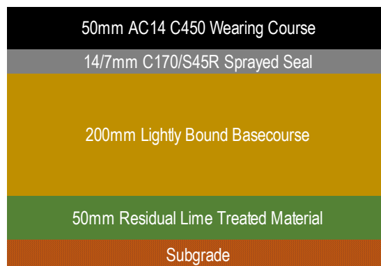
Figure 10: Pavement Design Cross Section [4]
