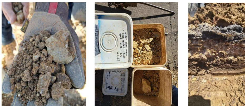
Figure 9: River Terrace Typical Materials
