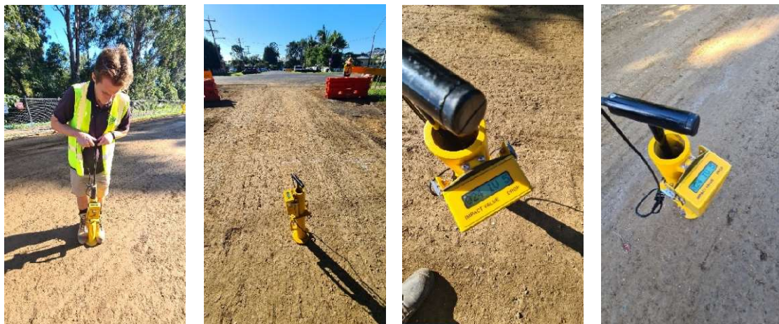
Figure 22: Clegg Hammer Testing
