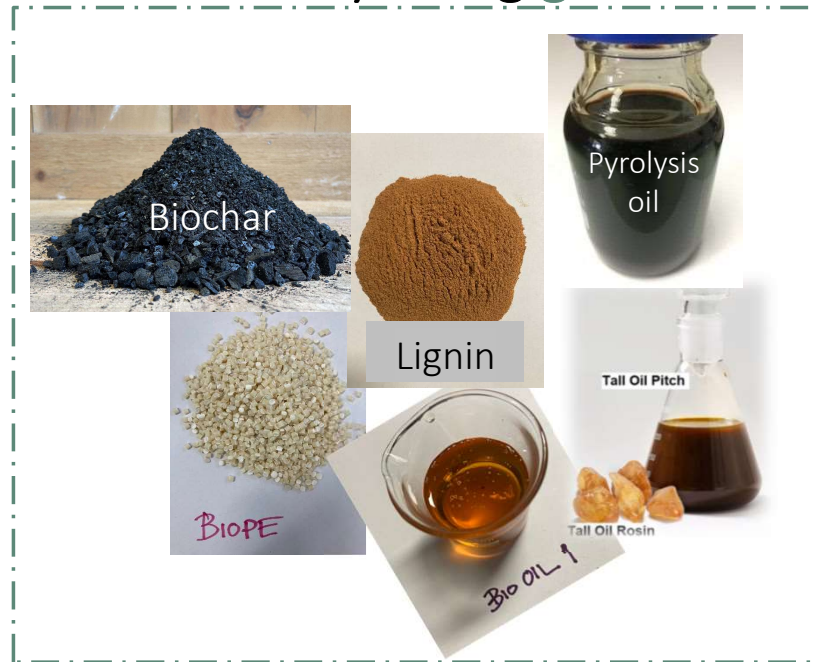
Example of possible plant based materials that can be used in Green Binders
