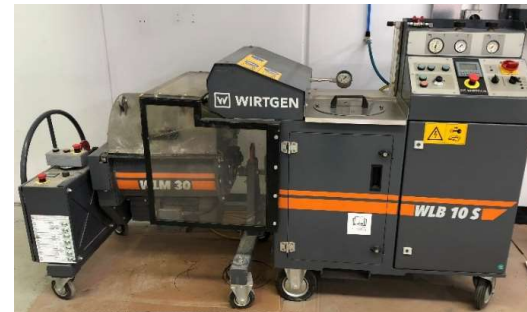
Mixing FBS material – Wirtgen apparatus
