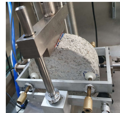
Indirect tensile modulus testing
