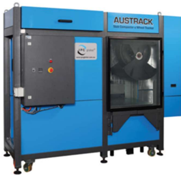
Austrack (Extra-large Wheel tracker)
