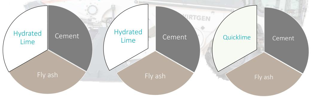
Linear Shrinkage >6 (40% Lime : 30% Cement : 30% Fly Ash) Linear Shrinkage <6 (30% Lime : 40% Cement : 30% Fly Ash)
