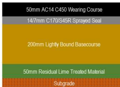
Figure 10: Pavement Design Cross Section
