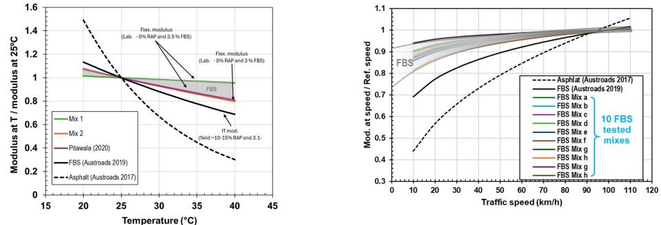
New flexural testing showed lower sensitivity to temperature and speed than currently assumed from past data
