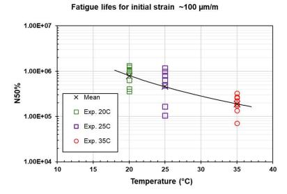
Effect of temperature on fatigue performance showed a drop in fatigue 4 to 5 times between 20 to 35 °C (based on two mixtures dataset) more that 50% lower than what academic research showed.
