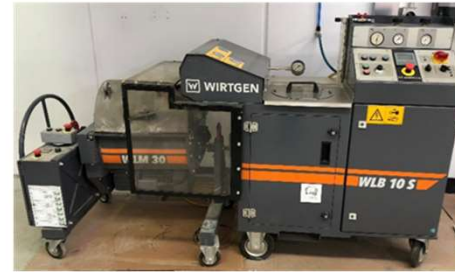
Mixing FBS material – Wirtgen apparatus
