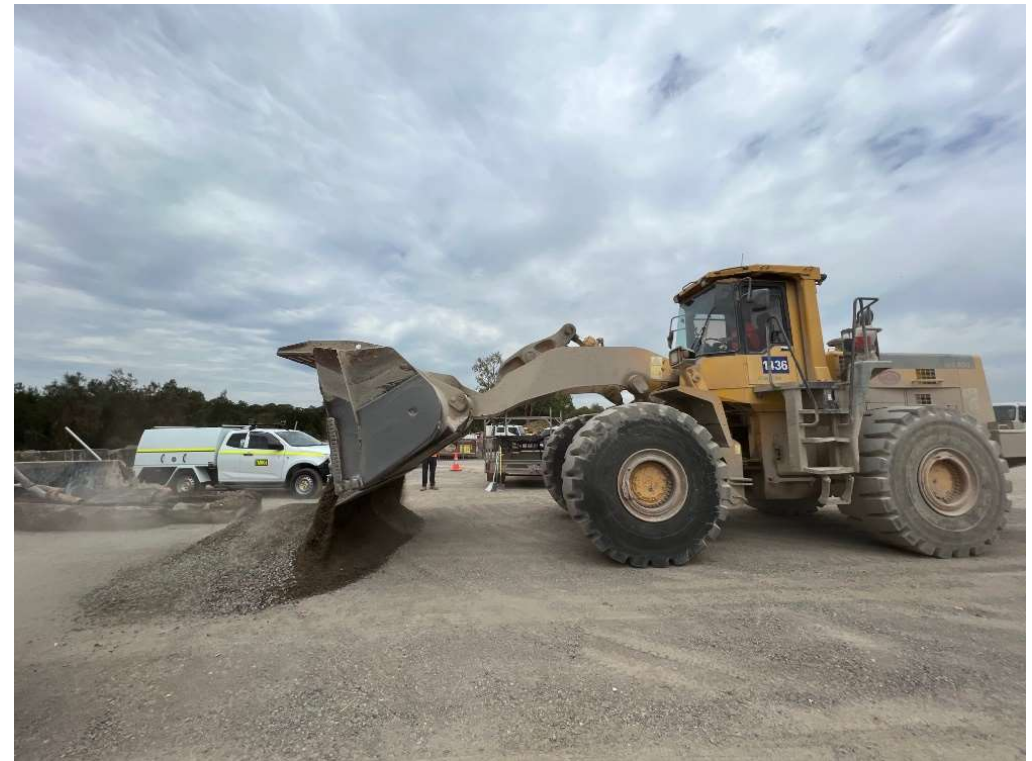
Material Sampling for TMR O24 Laboratory Testing
