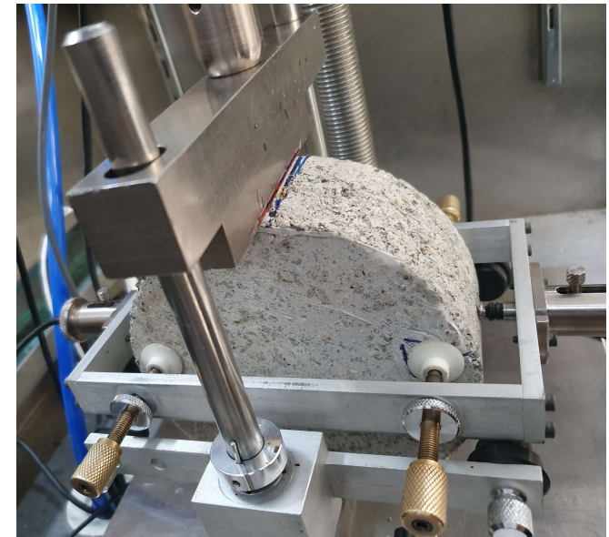
Indirect tensile modulus testing of FBS samples
