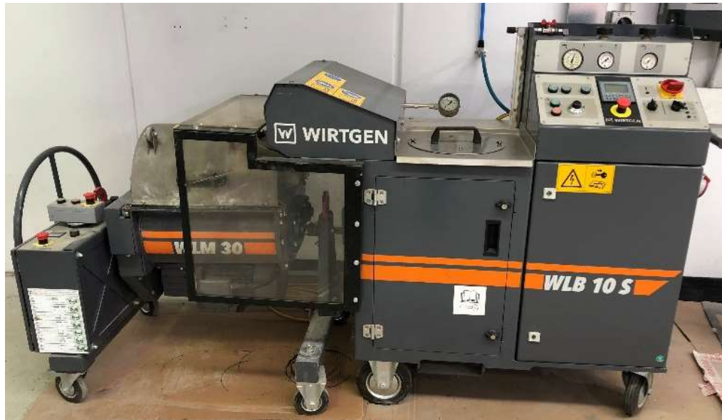
Mixing FBS material – Wirtgen apparatus
