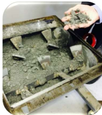
Foamed bitumen mix
