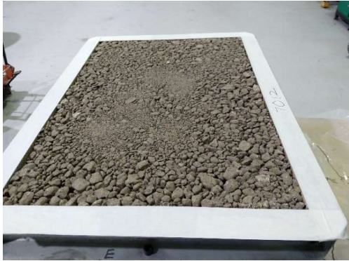
Surface after compaction
