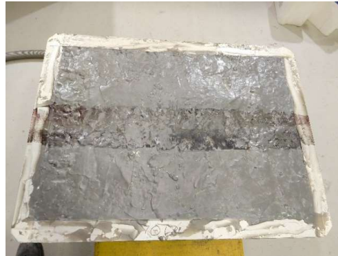
Sealed surface after wheel tracking
