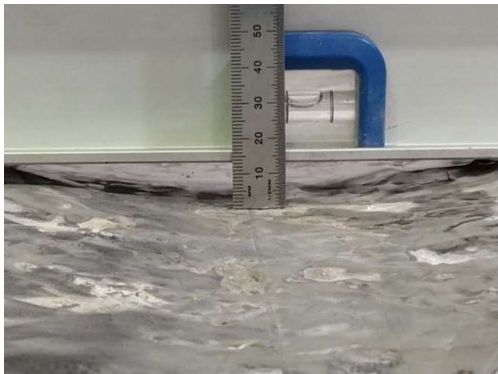
Sealed surface after wheel tracking
