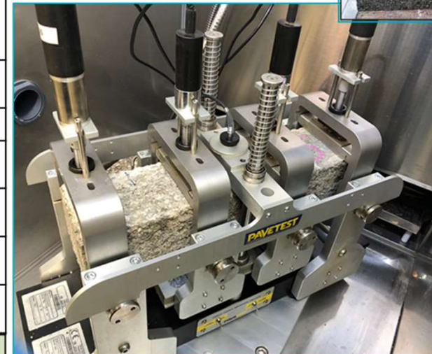
Four-point bending test
