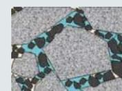
Bitumen coats the finer particles
