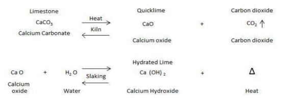
If hydrated lime is exposed to carbon dioxide, it may revert back to calcium carbonate
