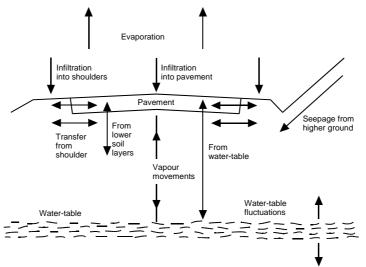
Figure 5 Moisture movements in road pavements (Austroads, 2004b)
