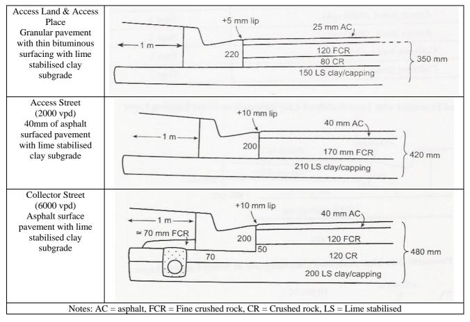
Figure 3 Standard pavement configurations incorporating lime stabilised subgrades designed by ARRB Transport Research for Wyndham City Council (Foley, 2000).
