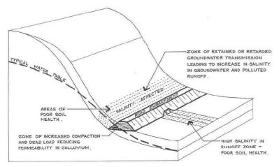
Figure 6 Roads and the pavement materials may cause an obstruction to moisture making its way down a hill (Porter, 2001).
