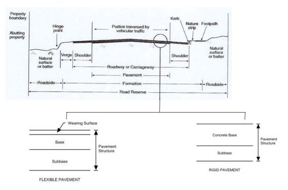
Figure 2 Road structures in the road easement (Dickinson, 1984).
