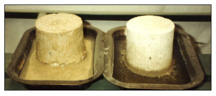
*Figure 5* A view of a pavement material sample unstabilised (left) and stabilised with DPP (right) subject to soaking in water for 24 hours.
