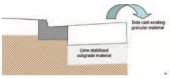
A. Existing pavement material is side cast to expose top of sub-grade. Depth of side cast material to include design depth of base-course stabilisation, an allowance for bulking due to volumetric change and an allowance for final wearing course thickness. Total bulking & wearing course thickness to be disposed.
