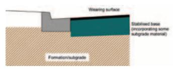
(b) Up to 30% of the subgrade could be used to stabilise a thin existing road.
