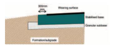
(a) Both base and sub-base materials are used to stabilise the road.
