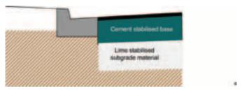
C. Construction of final wearing surface. Where a thin asphalt layer is to be the wearing course, it is recommended that a SAMI seal is used prior to placing the asphalt.
