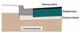
(a) Both base and subbase materials are used to stabilise the road.
