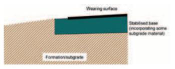
(b) Up to 30% of the sub-grade could be used to stabilise a thin existing road.
