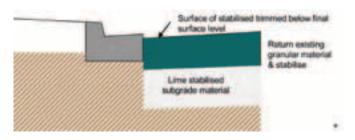
B. Cementitious binder is spread at specified rate and mixed to specified depth. Surface is trimmed below the lip of the gutter to allow surface treatment to be constructed after initial curing of pavement material.
