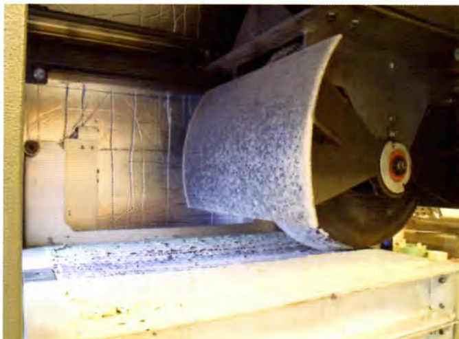
Austrack - A slab in tracking mode on the latest tracking equipment at ARRB Group.
