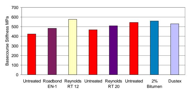
Figure 4 Basecourse Stiffness (Elmod back-calculated Resilient Modulus)
