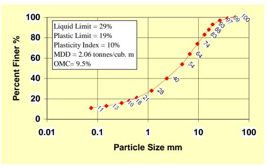
Figure 2 Sheeting Material Post Compaction Classification Properties
