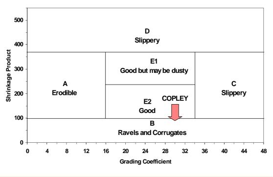
Figure 11 Grading/Plasticity and Unsealed Surface Performance<sup>[4]</sup>
