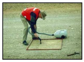
Figure 6 Removal of loose Surface Material
