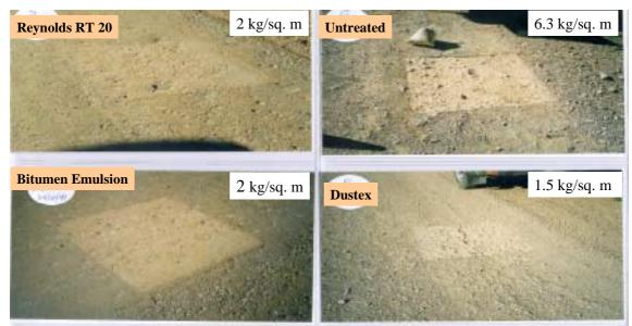
Figure 9 Pavement Condition after 450 days (June 1999)
