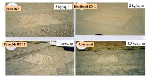
Figure 8 Pavement Condition after 450 days (June 1999)
