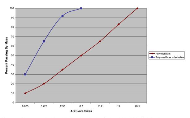
Figure 1 Recommended Particle Size Distribution for Insoluble DPP Stabilisation
