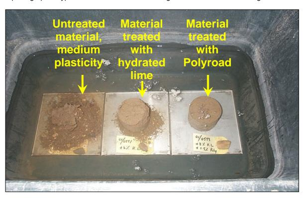
Figure 2 Capillary Rise & Swell Test AS 1141.53
