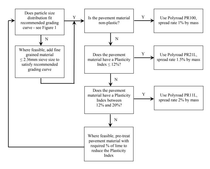
Figure 3 Mix Design Selection Flowchart
