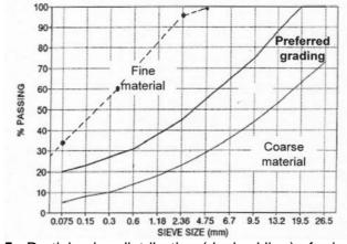
**Figure 5** Particle size distribution (dashed line) of prior stream gravel from SW region of NSW (Kok, 2003).
