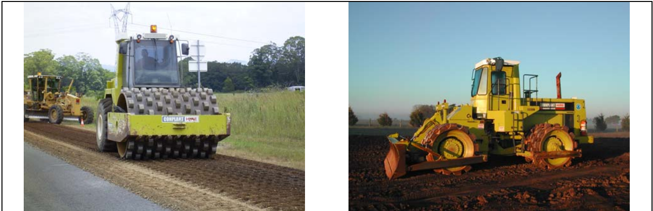
Figure 1 Self propelled vibrating (or static) 27 t padfoot roller (left) and soil compactor.
