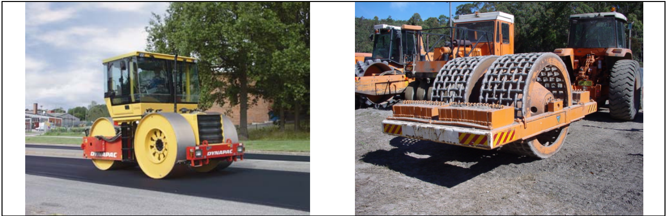
Figure 3 Typical three wheeled/point roller (left) and towed grid rollers are commonly used to break up macadam stones that have been incorporated in the stabilised base layer.
