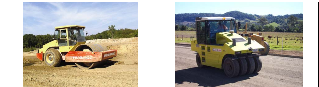
Figure 2 Self propelled vibrating (or static) smooth drum 15 t roller (left) and pneumatic multi-tyred roller.
