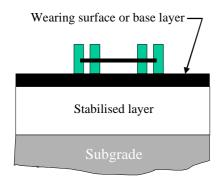
*Figure 1* A view of a typical cross-section through a stabilised pavement.
